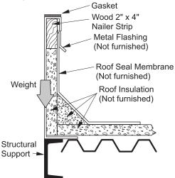
Each curb kit contains a hardware package. The package contains  $3/8-16 \times 1$ " bolts and nuts for assembly of the curb. Two  $1/4-20 \times 1/2$ " screws are included when the unit has a vestibule. Rolls of gasket are included to cover the top surfaces of the curb and supports.
